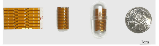
Fig. 5. The process of winding the FPCB Rx coil.
